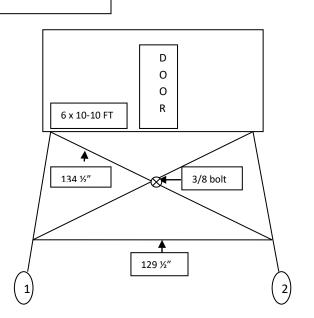
Install All Braces (Leave Loose) Set blind on Level surface
